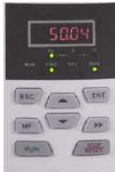
Fig. 4-7 Direct frequency modification status
