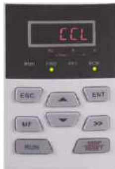
Fig. 4-4 Fault or alarm display status (CCL: Contactor act fault)
