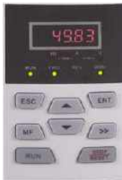
Fig. 4-6 Parameter value setting status (b0-02 is set to 49.83Hz)
