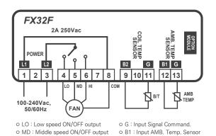
o B2 : Input COIL Temp. Sensor
